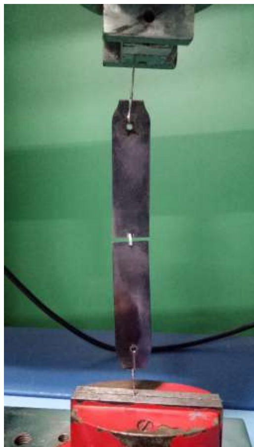
Fig 2: Microtensile bond strength testing in UTM
